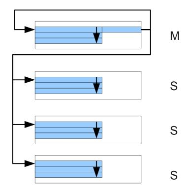
In Slave Crates S, CLK is input on the front panel LEMO to a local Master card which distributes to 2 slave cards using PXI.
